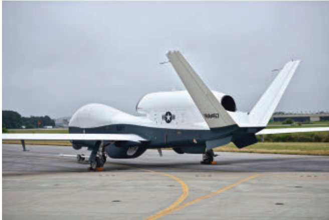
The Northrop Grumman MQ-4C Triton long-range maritime patrol unmanned aerial vehicle (UAV) is getting in on the electronic warfare game with a scheduled advanced signals intelligence package to enable the UAV to replace the manned EP-3 SIGINT aircraft.
